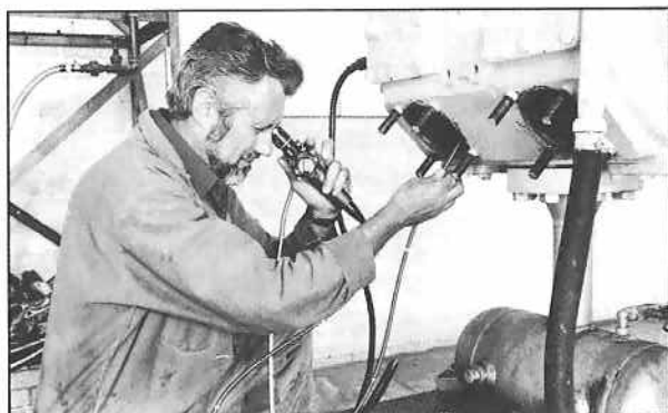
Olympus IF being used to inspect a reciprocating compressor
